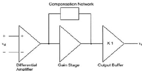
Fig. 2. Block Diagram of a generic amplifier.
