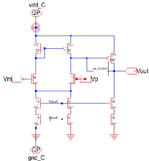
Fig. 3. Schematic for topology 1 for two stage operational amplifier.
