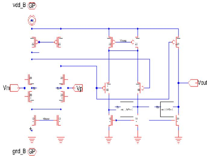
Fig. 7. Schematic for topology 3, two stage operational amplifier.
