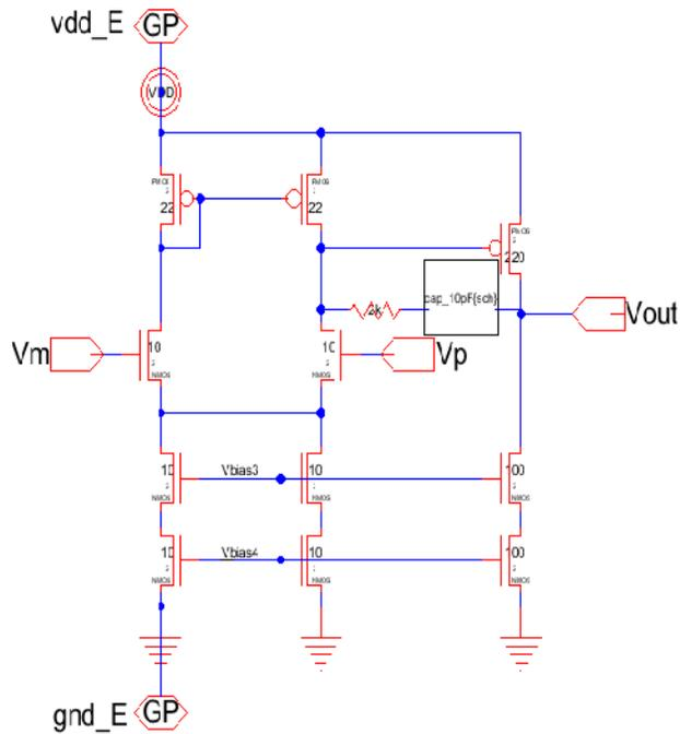
Fig. 4. Schematic for topology 2, 2 stage operational amplifier.
