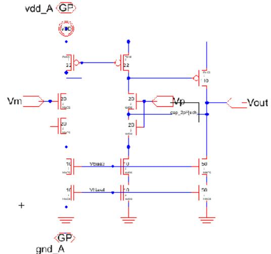
Fig.6. Schematic for topology 4, two stage operational amplifier.
