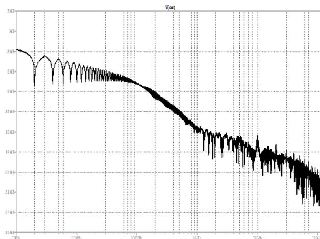
**Fig. 19. FFT Analysis plot for 3 stage CMOS Operational Amplifier.**
